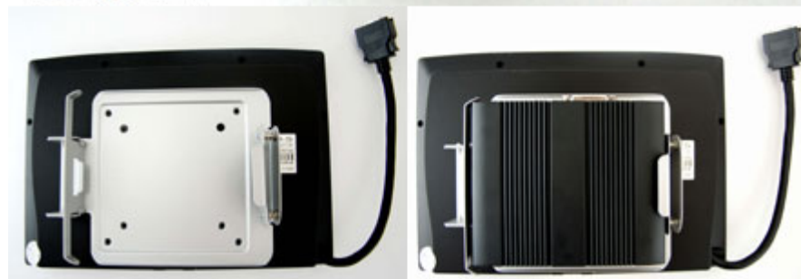
Example : QBOX mounted on CTF840-SH TFT display
